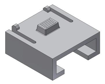
Notice that the part has features that are not relevant to our design analysis. Including these non-relevant features in the mesh would only increase the analysis time without any value.
