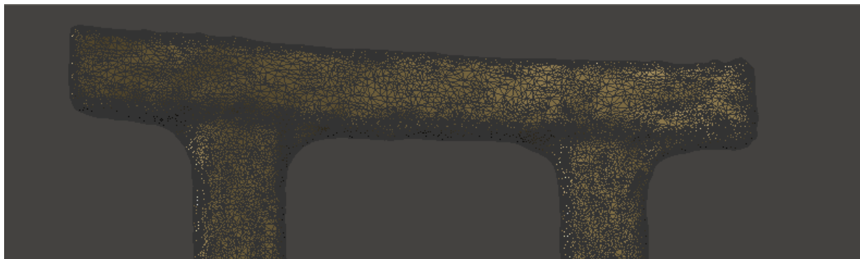
Figure 12 Image of Mesh Generated with Ultra Mode in Recap 360 (1660613 Triangles 830684 Vertices)
