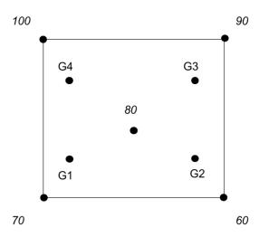
When two elements are connected together, we can start to understand how the post-processor needs to interpret the results.
