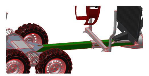
Just looking at a model like this, we can start to imagine some of the different things we need to think about before we begin our analysis. What type of analysis do we use? It can be static for understanding service loads and gravity or dynamic/transient if it is navigating difficult terrain or if logs are dropped into it. Should we use solid elements or shells or beams?
