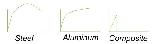
Even composites exhibit failure. However, when we perform a linear static analysis, we assume the material only operates in the linear range, or the stress/strain curve can be assumed to be linear.
