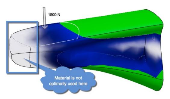
Smart Edit Form command offers automatic optimization of your model based on selected Edge(s)/Face(s). It moves it as far as possible to not to cause the model breakage.
