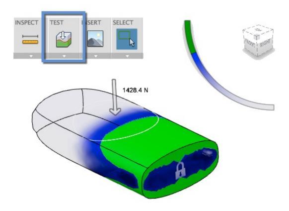
Modify the input by entering 1500 N (equals 150 kg) and move the load.
