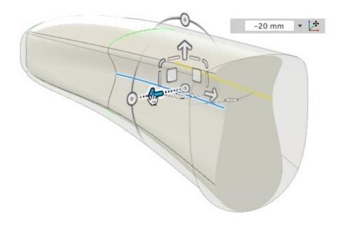
As a result, the modified design is better. The percentage of optimally used material is higher and the volume decreased from 122 cm<sup>3</sup> to 76 cm<sup>3</sup>.
