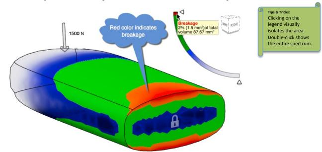
For load of 150 kg, the current design fails. The red area indicates breakage.
