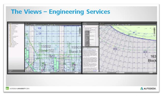
Engineering precision mapping capability - Showing the underground services within a specific area as well as the Level information. Quality Codes provides guidance as to the accuracy of the information which is critical in such a highly sensitive area to undertake construction/works.
