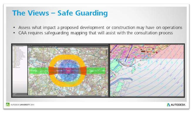
Horizontal and Conical Surfaces, Approach and Take-off Contours and Radar information, ILS sensitive Areas.
