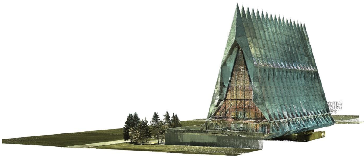
Point cloud generated by laser scans performed by USAF, as displayed in Revit
