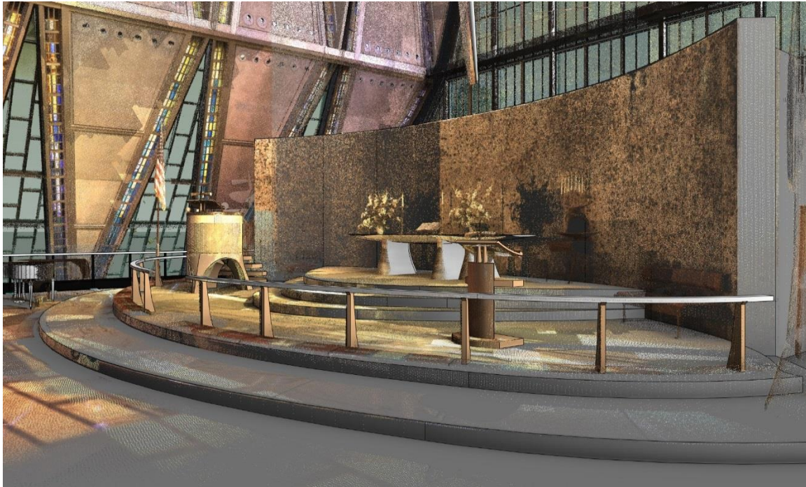
Revit model showing elements in sacristy derived entirely from the point cloud
