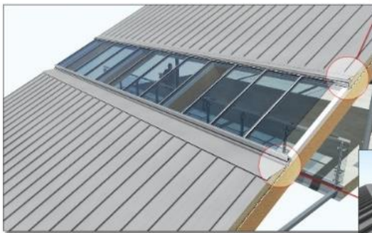
Kings Cross Eastern Goods Yard re-development Eastern Transit Shed proposed glazing details
