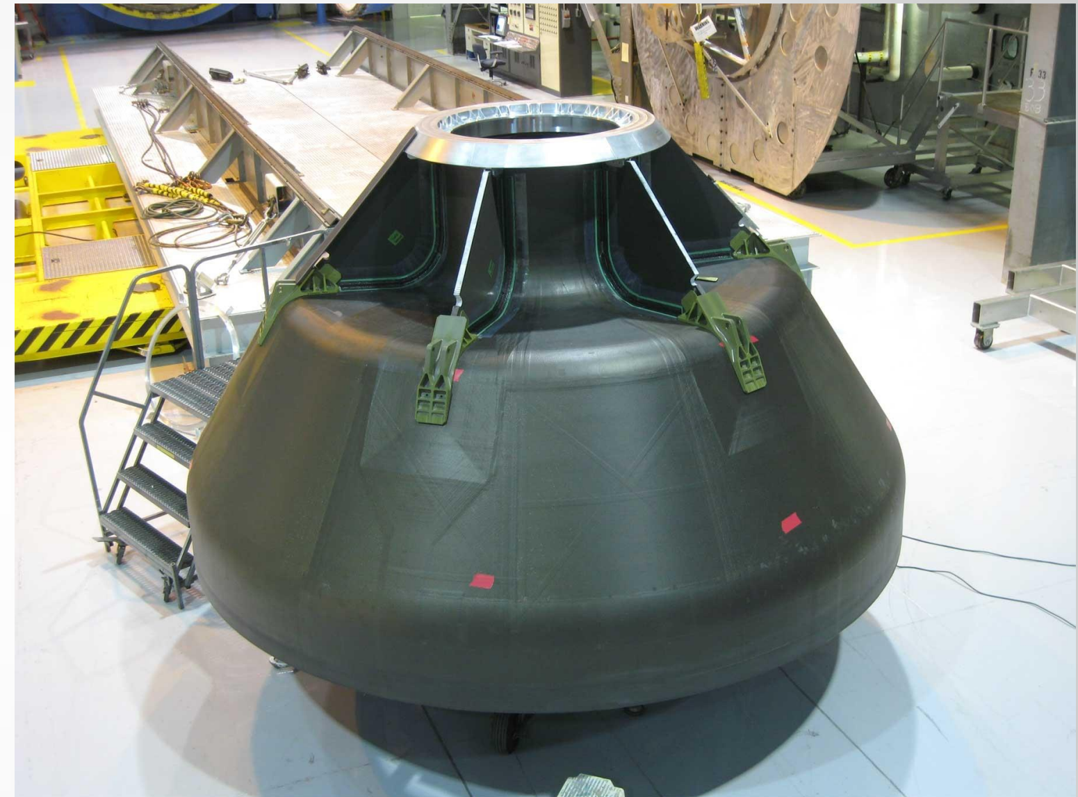
Composite Crew Module (Image: NASA's Langley Research Center)
