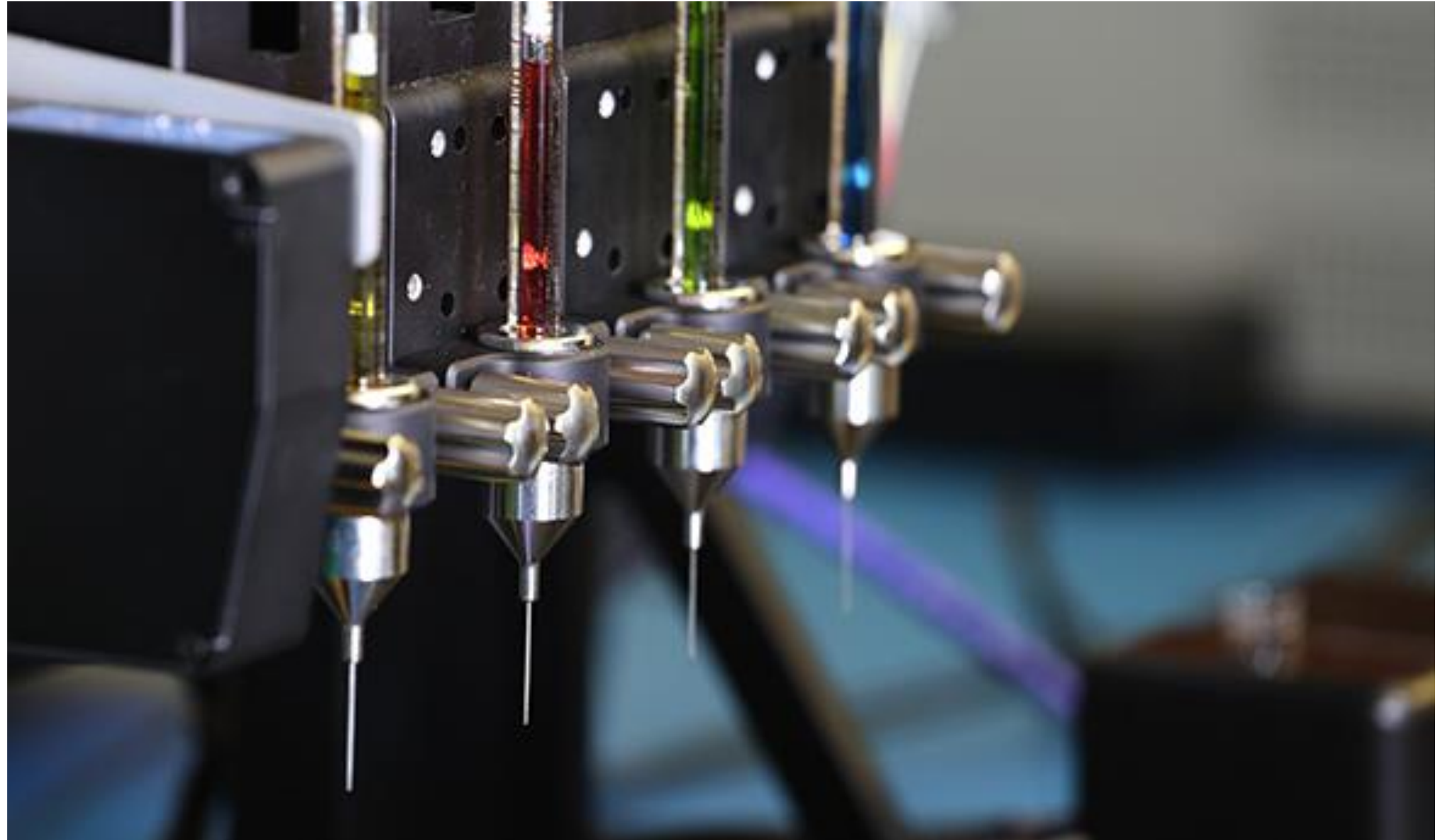
Organovo's NovoGen Bioprinter fabricating tissue.
