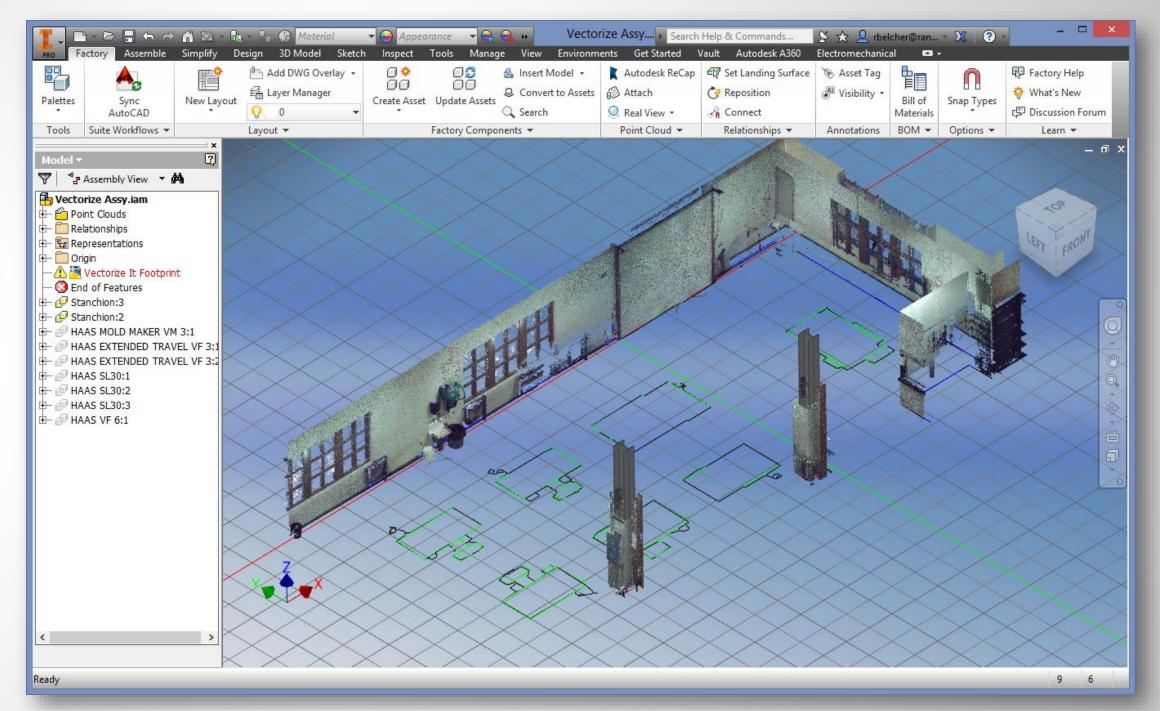
The extracted section lines are used as a DWG overlay in FDS.
