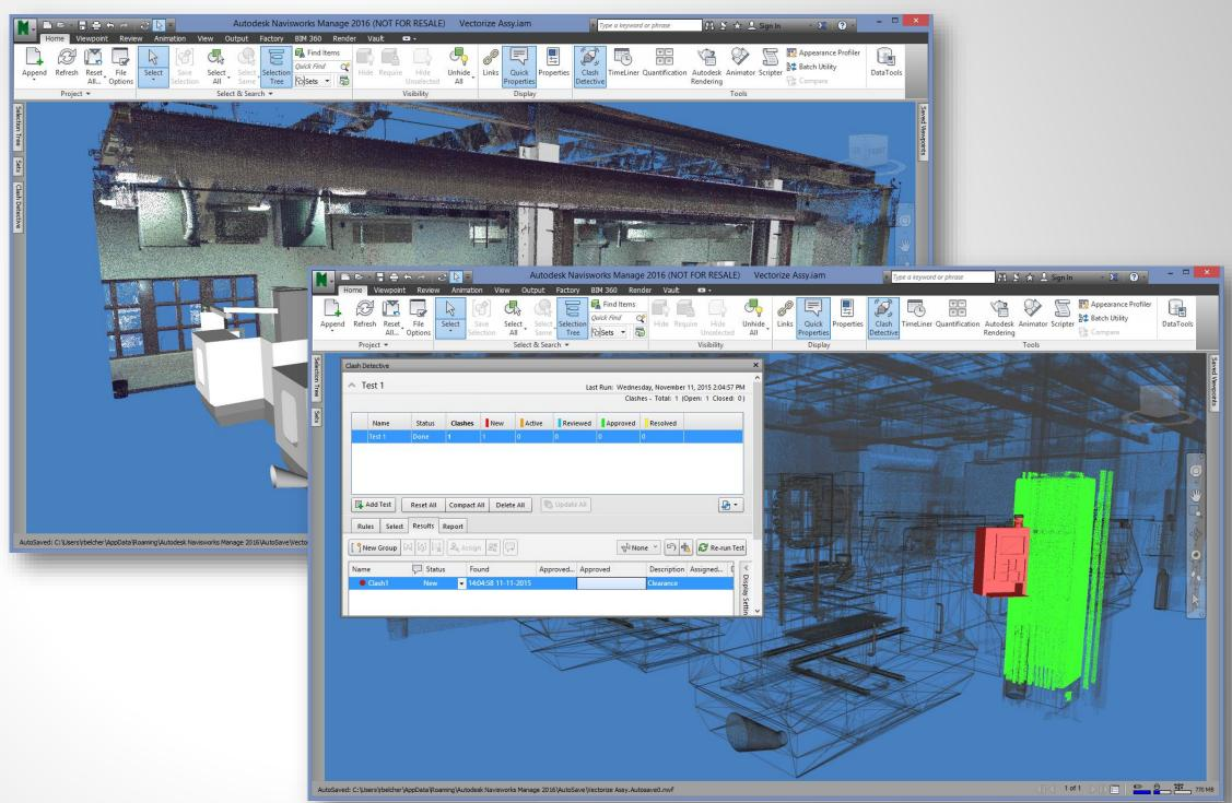
Analyze the digital assets in way of the Point Cloud - Clash Detection
