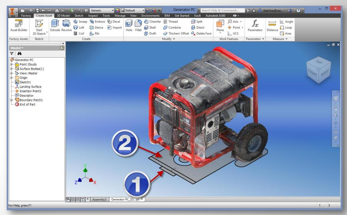
Add additional sketches and surface patches so the asset functions correctly in Inventor, Navisworks, and AutoCAD.
