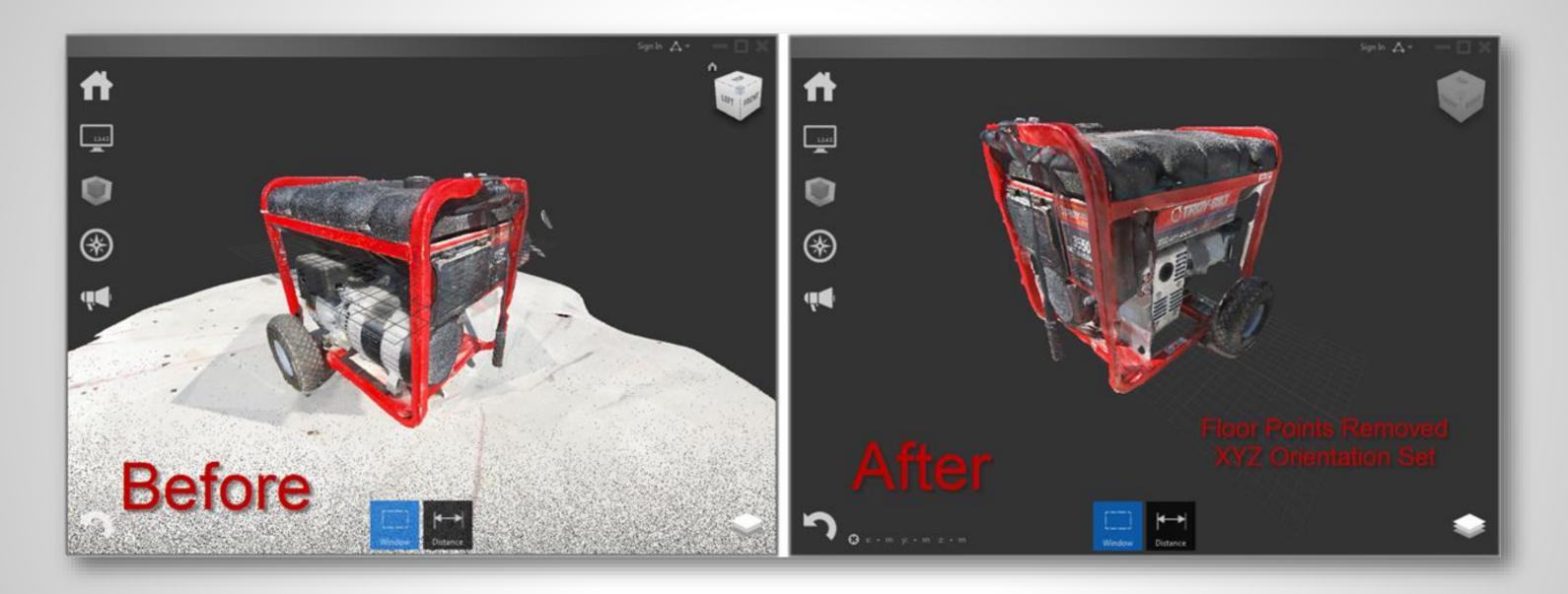
Use ReCap to orient the scan and remove any point that is not part of the asset.
