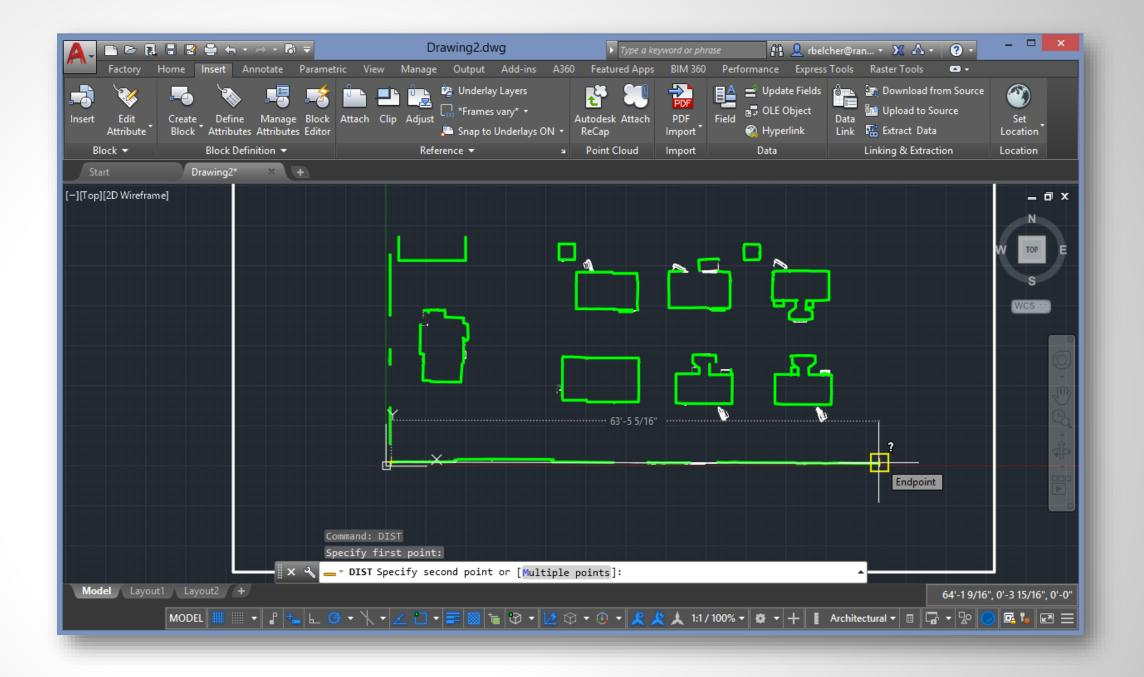
Add a dimension value to scale the vector geometry correctly.
