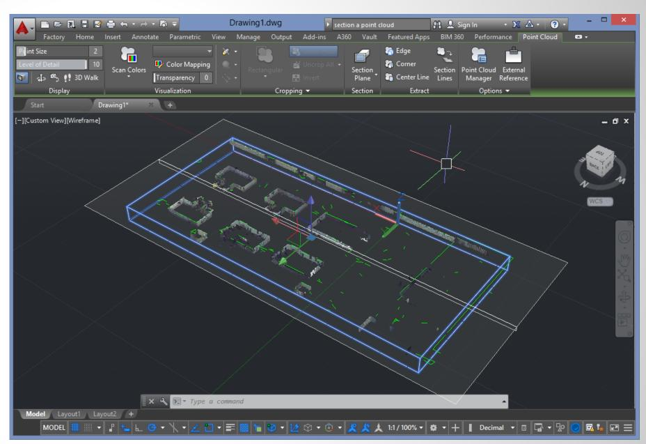
AutoCAD offers a number of geometry extraction tools for Point Clouds.
