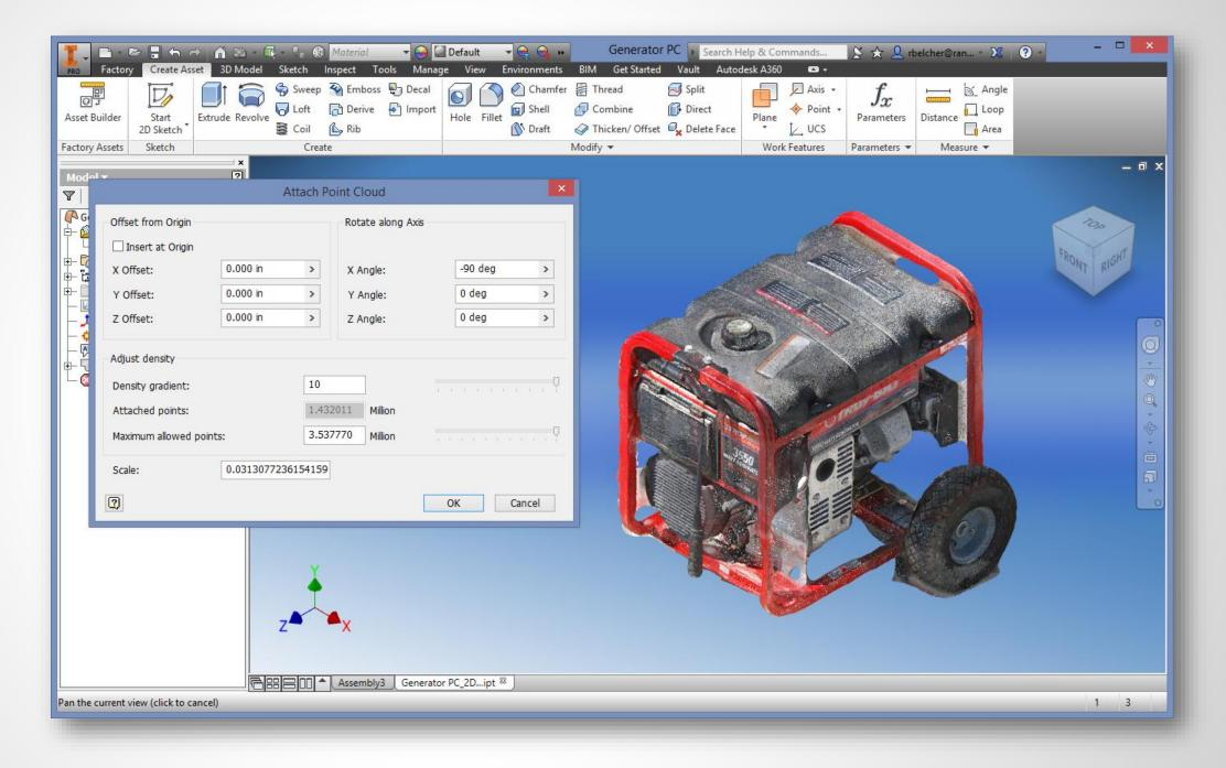
The Orientation set in ReCap is honored when placing the scan into Inventor.
