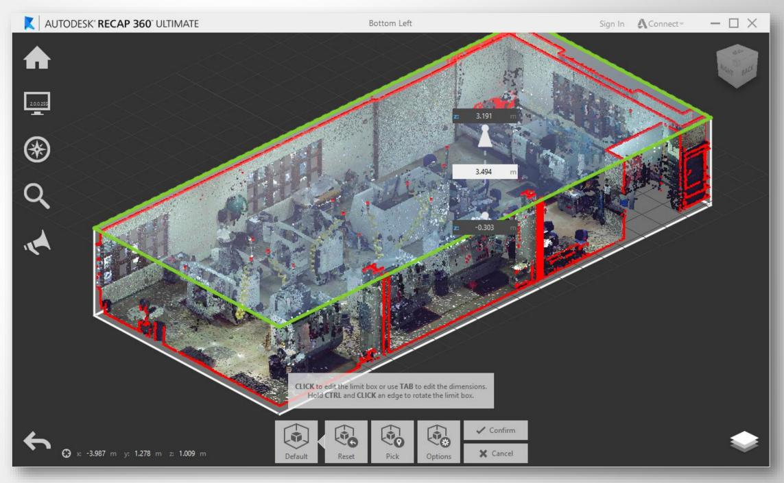
Temporarily remove points to access the interior of the scan.
