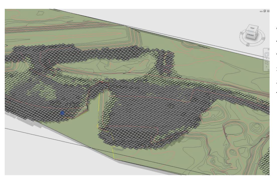
Now for the next example we are going to show how to take the slab flatness workflow and take it one step further to comparing to a designed elevation rather than a planar elevation.
