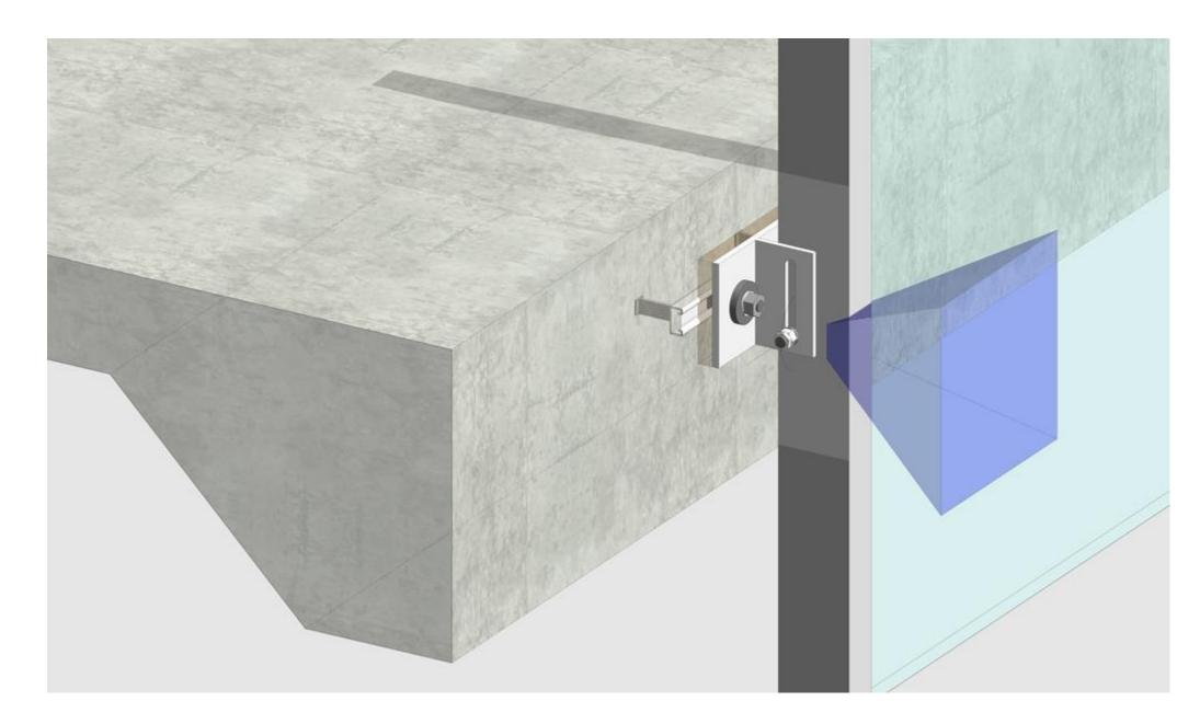
Moves up-down, left-right and in-out of plane. As the contractor we are required to place the halfen channel and slab edge in the desired location plus or minus our specified tolerance. This shows how the connection "absorbs" those tolerances
