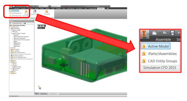
This tool will start the Simulation CFD software and request a name for the simulation's Design and Scenario. The Study name is already the same as the Inventor file that the study was launched from.
