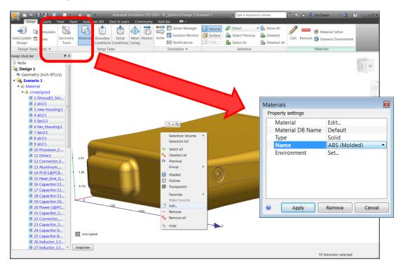
A useful technique when manually applying materials is to apply the material, then hide that object. This makes it easy to pick the next object on the screen.
