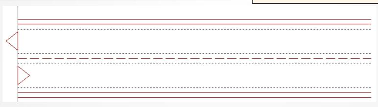
Traffic loads occupy a loaded width of 10ft within the lanes and will be located transversely so as to produce the most adverse effect
