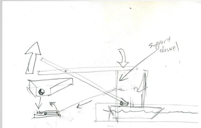
Initial design concept based on single ball bearing impact
